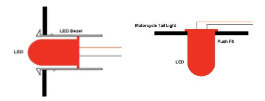
The LED with Bezel may be mounted through an inner fairing panel or even mounted through a light lens into a tail light unit. Warning: When fitting into an LED tail light take care not to damage the internal rear light circuit board.
