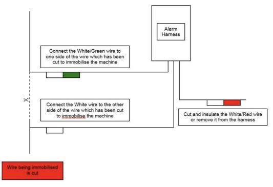
Important notice: On CANBUS based machines it is recommended that the only circuit cut is the wire between the kill switch and the ECU. Other points of immobilisation are likely to create fault codes. Most CANBUS based machines are equipped with a transponder immobiliser as standard
