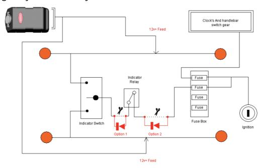
If you are unsure which way to fit the diode, cut the selected wire; hold the diode in line and with the ignition on set the indicator to the left or right. If the indicators work normally, you have got it the right way round. If they do not operate, reverse the diode and test again. Once you have it the right way round, solder it in line and protect the joints with heat shrink or good quality tape.
