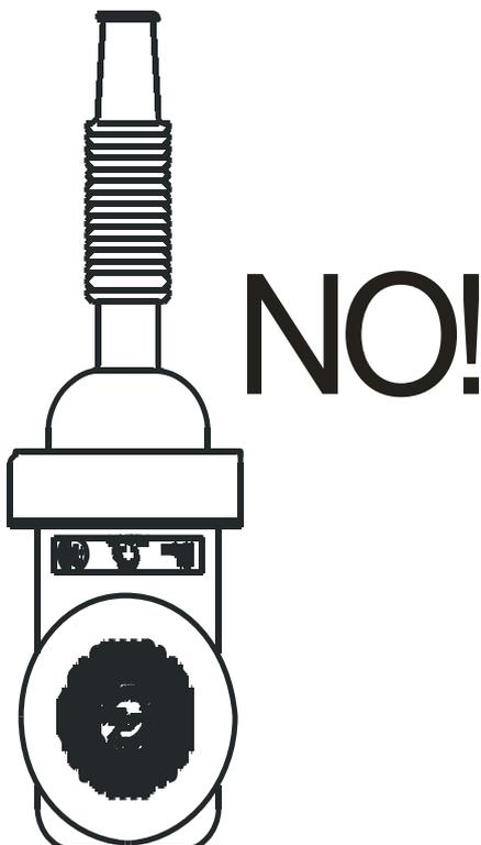
**Do not** install the alarm unit in this position as water ingress over time may seep through the rubber sheath and permanently damage the electronic circuit making the alarm system unreliable.
